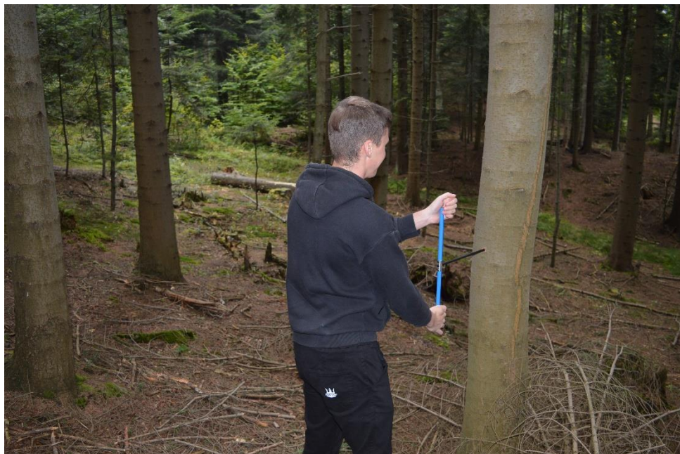
Photo. 11. A high school student drilling a tree core using a Pressler borer during a field workshop
